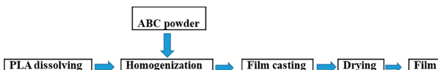
Figure 4. Stepwise fabrication process of ABC/PLA composite film.
